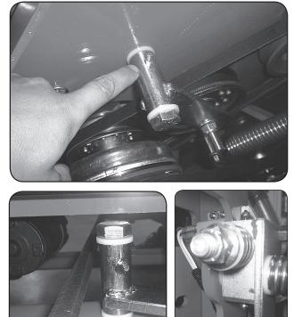
free of the pulley. Exercise caution while performing this step as fingers can easily become caught between the belt and pulley. For optimal cutting performance, the blade enclosure should be level from right to left and have a slight
