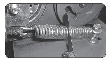
Factory setting is about .030  $^{\prime\prime}$  (about the thickness of a credit card) between coils as shown.
