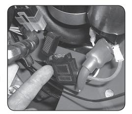
Always check the condition of the wiring harness ground cable. Ensure that the ground is connected, clean, and tight.
