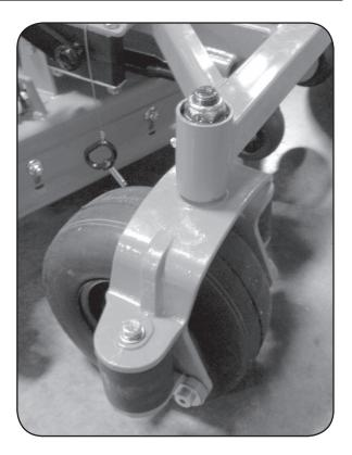
Torque rear wheel lugs to 65-75 ft. lbs. Re-torque at every oil change and check at every mowing.
