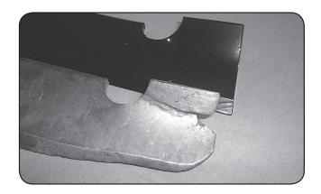
To change blades, it may be easier to use a piece of wood to keep the blade from turning so that the bolt can be loosened. **Bolts used have right-handed threads.** Retorque the blade bolts to 90-110 lbs. The blade spindles contain two sealed ball bearings inside the top and bottom of the spindle. The bearings are replaceable for a more cost effective repair.
